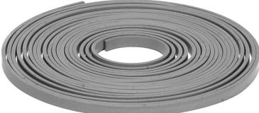
These are high performance engineering thermoplastic material consisting of PTFE and Sintered Bronze having properties of self-lubrication and wear resistant suitable for operating temperature up-to 260 degree centigrade. These are widely used in machine tool OEM's and maintenance / reconditioning and retrofitting of machines like milling machines, machining centers, SPM, Lathes, Grinding Machines, CNC Machines and many more for avoiding metal to metal contact.
